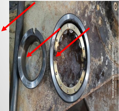
Damaged Bearing – after removing using gas cutting 3
